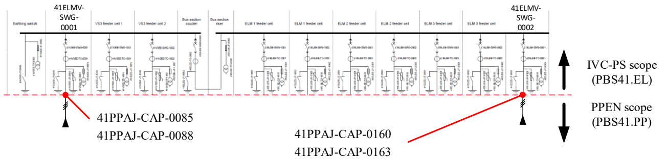
Figure 2. Conceptual schematic of the ELM power supplies system (from [RD1]).
